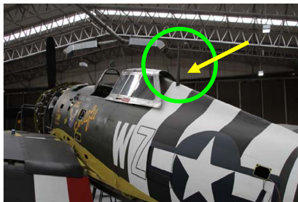
The antenna mast on this P-47G is off-set to the left
